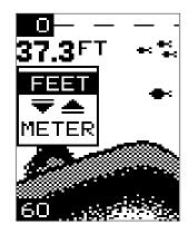
To change from feet to meters or vice-versa, press the menu key until the FEET/METER
